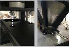
ULTRA-600 only: With the drop tube and vacuum chamber fill valve securely in place, slide the recollector between the frame legs and install onto the threaded rods of the fill valve, located underneath the heating hopper.
