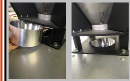
ULTRA-600 only: Install the **vacuum chamber fill valve** to the underside of the heating hopper using the supplied hardware  $(3/8"-16 \times 1")$  flanged hex bolts). The air cylinder must be on the BACK SIDE of the machine.
