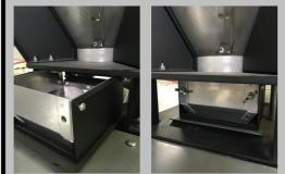
If equipped with the (optional) level sensor, attach it to the level sensor column mount at the top of the heating hopper, as shown.
