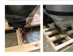
The heating hopper is secured to the pallet using four bolts (1/2"-13 x 2.5").
