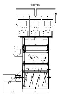
Compartments 1 & 2 - 4 cu ft [112 Litres] Compartments 3,4,5 - 3 cu ft [84 Litres]
