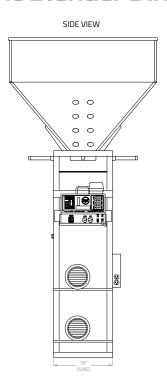
Compartment 1 - 6.6 cu ft [185 Litres] Compartments 3 & 4 - 3.3 cu ft [92 Litres] Compartments 2 & 7 - 2.5 cu ft [70 Litres]
