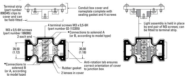
1. For DC coils the +ve lead(s) must be connected to the terminal(s) marked +. When using 3-wire incom-
