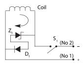
NOTE: These surge suppression devices are "Polarity Dependent." Proper biasing conditions must be met when installing/connecting a coil in a system. Times represent cessation/application of voltage to coil versus velocity (start/stop) of a cylinder using a single solenoid, spring offset valve (time in milliseconds).
