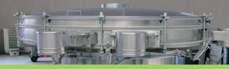
EA variable and easy selection of screen inserts with only a few fasteners, allows a fast adjustment to changed process conditions from 2 to 7 fractions within one machine with maximum screening efficiency.
