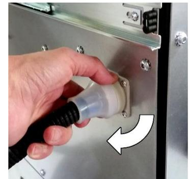
Slide the Retention Hopper sealing collar up so that the magnets engage onto the bottom of the Vacuum Chamber.
