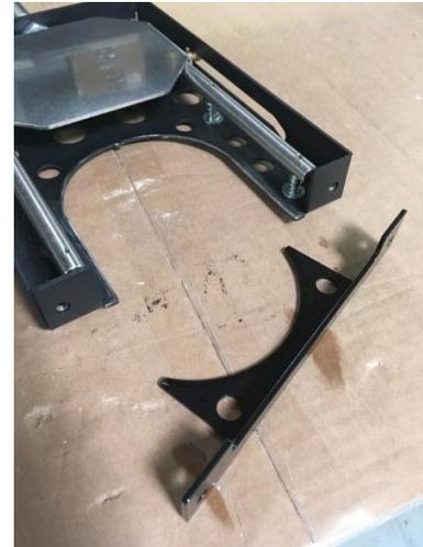
Insert the upper vacuum slide gate assembly into the groove of the mounting collar on the vacuum chamber tank head.
