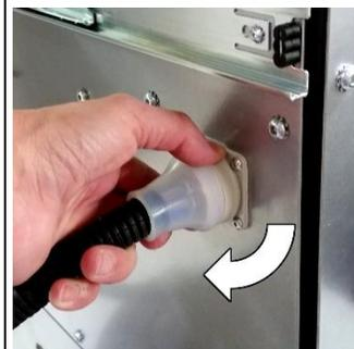
Turn on air pressure. Rotate counterclockwise.
