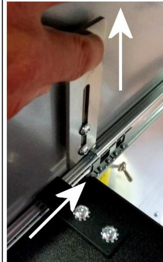
Push the Slider rails and Vacuum Chamber back into the Dryer until the Slider Lock falls into place in front of the Vacuum Chamber Slider, locking the Vacuum Chamber Slider into the operating position.
