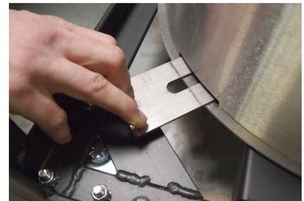
At the base of the Retention Hopper are two slots that must be aligned with the locator bolts.
