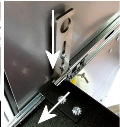
Rest the Vacuum Chamber onto the fully extended Sliders. The Vacuum Chamber has three resting pins. Orient the side with two resting pins on the left Slider rail.
