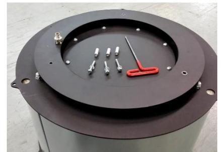
Remove the three black plastic plugs located on the upper plate of the Heating Hopper. See photos.
