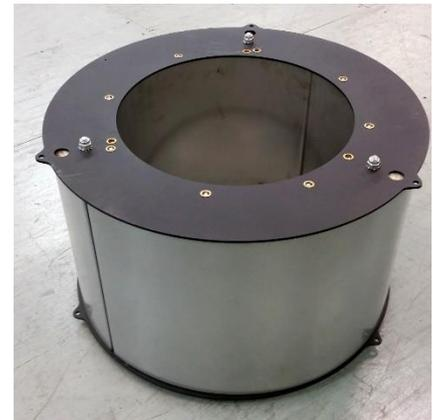
Remove Loader Adapter Plate / Diffuser Assembly from the top of the Heating Hopper by removing the three 1/4-20 button head screws and spacers. Lift the Loader Adapter Plate off of the Heating Hopper.
