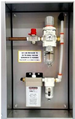
Air pressure affects the ability to draw a high vacuum. We recommend a pressure setting of **85 PSI while the dryer is resting idle**. Air is used when the **vacuum generator** is running so observe the PSI while the Dryer is drawing a vacuum. The gauge should continue to read this setting even when the vacuum unit is on. If it does not maintain pressure your supply line is not sized properly.
