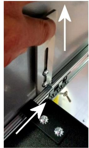
Push the Slider rails and Vacuum Chamber back into the Dryer until the Slider Lock falls into place in front of the Vacuum Chamber Slider, locking the Vacuum Chamber Slider into the operating position.
