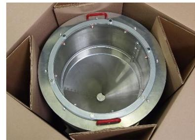
Close the slide-gate to allow the Retention Hopper to seat down onto the base of the ULTRA-150/300. Once seated open the slide-gate to allow material to flow.
