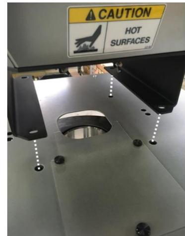
Using a 9/16" open-end wrench and ratchet, secure the heating hopper to the machine using the mounting hardware that was provided. Tighten down firmly.
