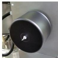
Remove wing nut and slide off filter housing and filter.
