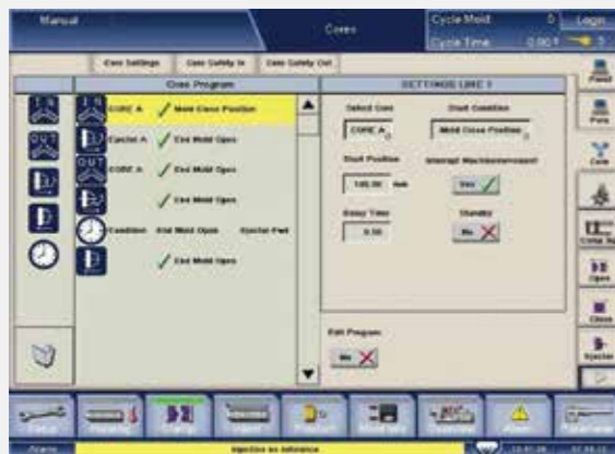
New flexible core sequence.
